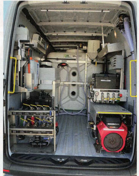
Green Pro's Sprinter spray van carries all of the spray and injection gear, along with multiple tanks and 500 gallons of water. Photo courtesy of Green Pro.
