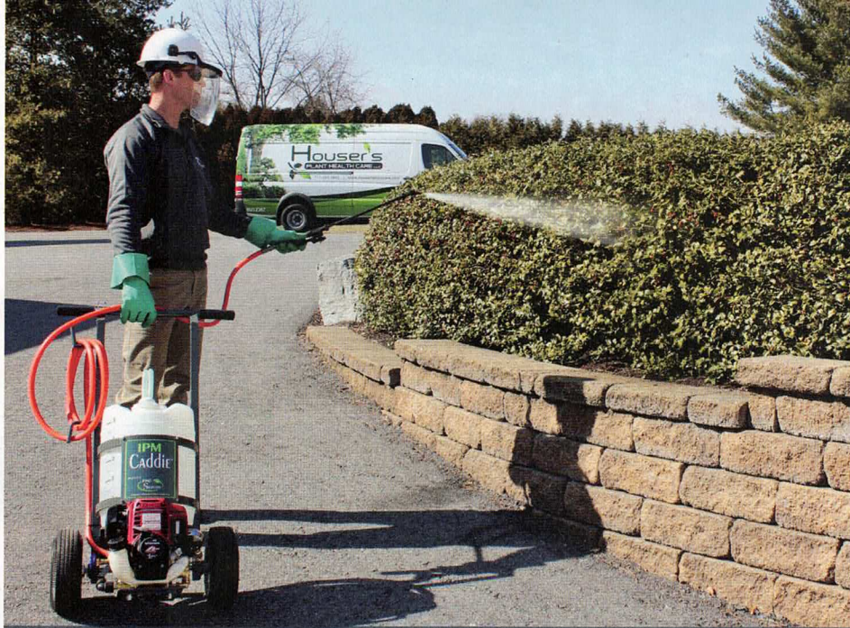
The IPM Caddie is a wheel-mounted, portable spray system that includes a gas-powered pump and loader. "It's almost like the backpack, but it's on wheels," says Bob Houser. Photo courtesy of Bob Houser.
