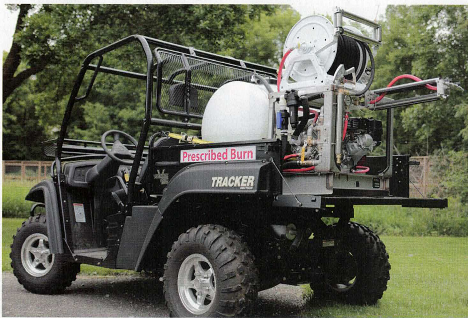
Altec's SK55 is one of its small, skid-mount sprayers that come in sizes from 55 to 110 gallons. They are commonly used for pest control, burn control and right-of way-applications. Photo courtesy of Altec Spray Equipment.
