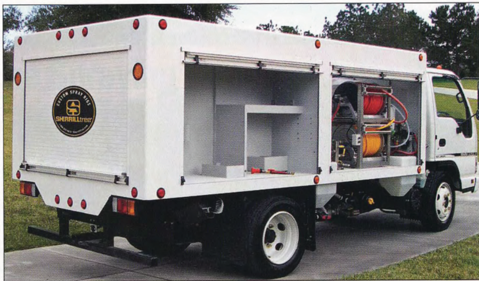
The equipment needed to apply compost tea, which when brewed is good for 12-14 hours only, needs to be low-maintenance and relatively easy to use, says SherrillTree's Tom Duffy. SherrillTree provides corrosion resistant all aluminum bodies with stainless steel fully balanced diaphragm pumps for contamination free compost tea applications.
