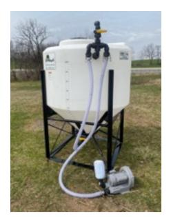
**Assembly Instructions:** Please note that the components are designed to be assembled one way only. The air blower hose is connected to a fitting at the top of the tank. The other hose goes from the other side of the connection to the bottom of the tank. This is a safety feature designed to minimize the chances of liquid getting into and damaging the blower due to an electrical outage.
