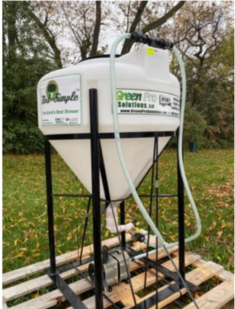
1. Before starting the blower, ensure that both the air valve and the drain valve on the bottom of the tank are in the off (closed) position, so that the valves are at right angles to the fittings.
