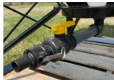
2. Connect one hose to the fitting on the bottom of the tank. The other end connects to the fitting at the top of the tank. The second hose attaches to the blower at one end and the top of the tank. Use the appropriate length if the hoses are different lengths. Now the air will flow from the blower, through the air check valve and on to the bottom of the tank. Air will not flow into the top of the tank.
