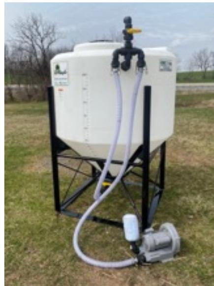
**Assembly Instructions:** Please note that the components are designed to be assembled one way only. The air blower hose is connected to a fitting at the top of the tank. The other hose goes from the other side of the connection to the bottom of the tank. This is a safety feature designed to minimize the chances of liquid getting into and damaging the blower due to an electrical outage.
